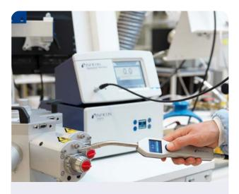
The TGF11 is an accessory to INFICON hydrogen and helium leak detectors. It is a stand-alone unit which allows for easy and reliable tracer gas filling and evacuating.
