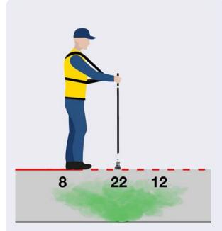
Press the bell probe against the ground and draw samples. The highest measured concentrations indicates where the traditional bar holing should be initiated.
