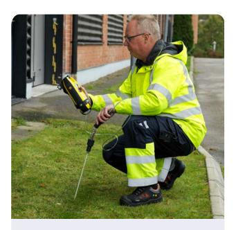
Bar holing is a method of measuring gas concentrations on a defined depth below the ground surface, in order to determine the location of the leak.
